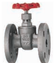
Van cửa ty chìm Inox 304 nối bích JIS10K Fig. UEB Stainless Steel SCS 13 Gate Valve Non-Rising Stem Flanged Ends JIS10K DN15A - DN80A
