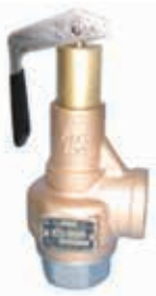
Van an toàn đồng có tay nối ren 0.05 ~ 1.0MPa, Model AL-150L Bronze Safety Relief Valve Screwed End Size DN15 - DN50
