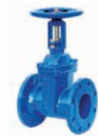
Van cửa gang dẻo ty nổi bích PN16RF, phủ sơn Epoxy, Ductile Iron OS&Y Resilient Seated Gate Valve, Flanged Ends PN16RF DN50-DN600
