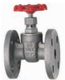
Van cửa ty chìm Inox 304 nối bích JIS10K Fig. UEB Stainless Steel SCS 13 Gate Valve Non-Rising Stem Flanged Ends JIS10K DN15A - DN80A
