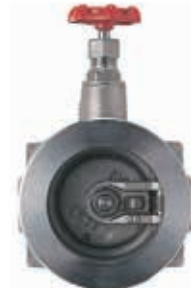
Van 1 chiều lá Inox 304 nối bích JIS20K Fig. 20UOA Stainless Steel SCS13 Swing Check Valve Flanged Ends JIS20K DN40-DN450
