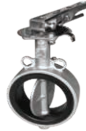
Van bướm gang đúc tay quay JIS10K Đệm kín EPDM/NBR Cast Iron Butterfly Valve JIS10K - Gear Type Seat EPDM/NBR DN50A - DN600A
