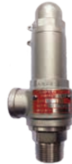
Van an toàn Inox không tay nổi ren 10kgf/cm 2 Model L9SP Stainless Steel Safety Valve 10kgf/cm 2 Screwed Ends - No Lever DN15A - DN50A
