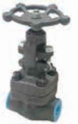
Van hơi thép rèn A105 nối ren Class 800 Forged Steel A105 Globe Valve Screwed Ends Class 800 DN15A - DN50A
